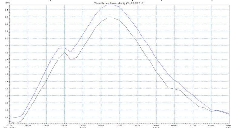
Figure 6. Changes in flow rate for 25-year-old flood at location of spur No. 3 (Blue line is with spur – Black line is without spur)
