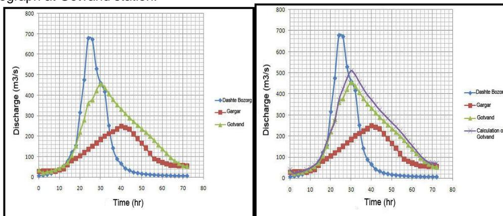
Figure 3. Comparison of simultaneous observed and computed hydrographs in Gotvand station for accuracy assessment in 12.14.1999.
