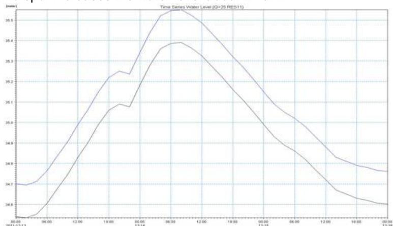
Figure 5. Changes in water level for 25-year-old flood at location of spur No. 3 (Blue line is with spur – Black line is without spur)
