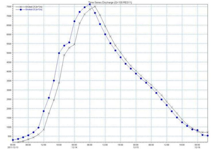
Figure 4. Comparison of the flood hydrograph with 100-year return period in Shoteyt River considering the spurs (blue and black lines are before and after flood hydrograph in before and after the spur location, respectively)
