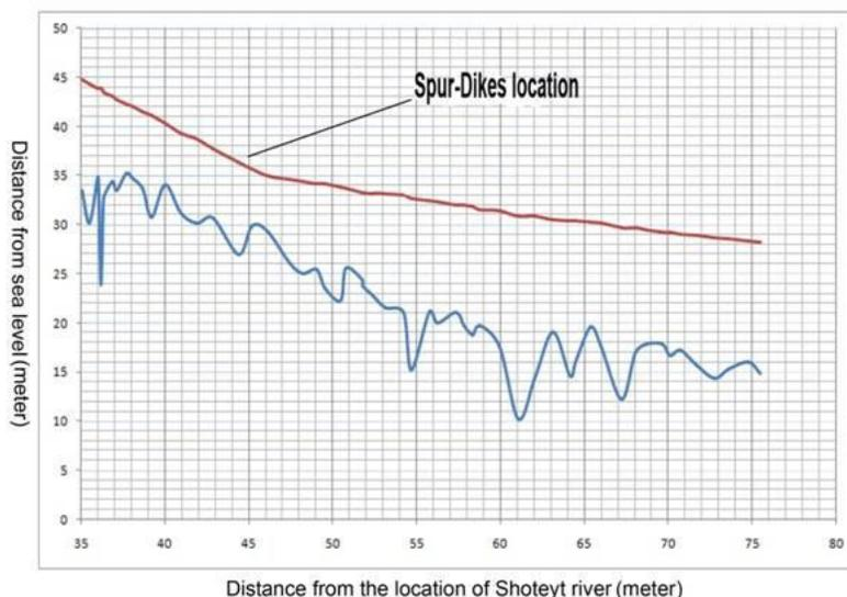
Figure 1. Longitudinal profiles of Shoteyt River for a flood with return period of 100 years (red line is water level – blue line is the digits of river bed).
