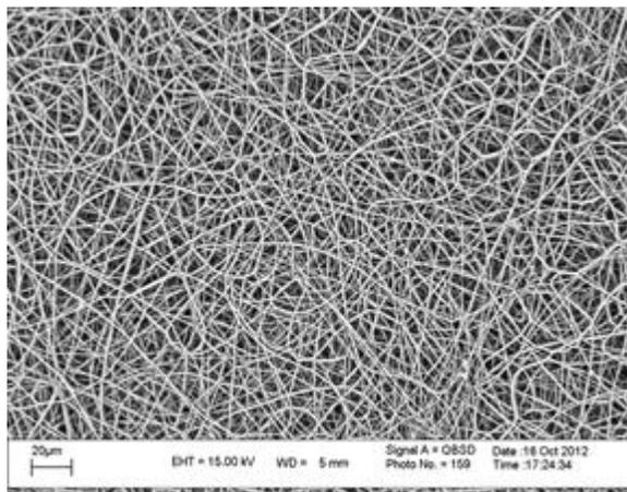
Figure 3. scanning electron microscopy image from PLLA nano-scaffold (500X)
