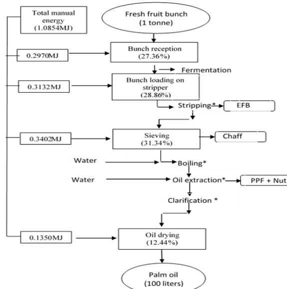
Figure 1. Flow chart for the processing of palm oil by semi-mechanized processor in Bayelsa state, Nigeria (\*= operational activities that do not require manual energy)
