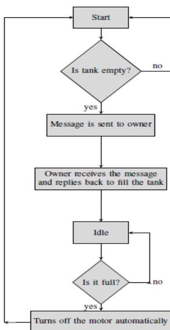
**Figure6:Use of GSM motor**
