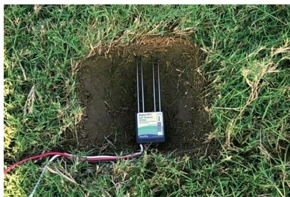
**Figure 2: Soil moisture sensing in field**
