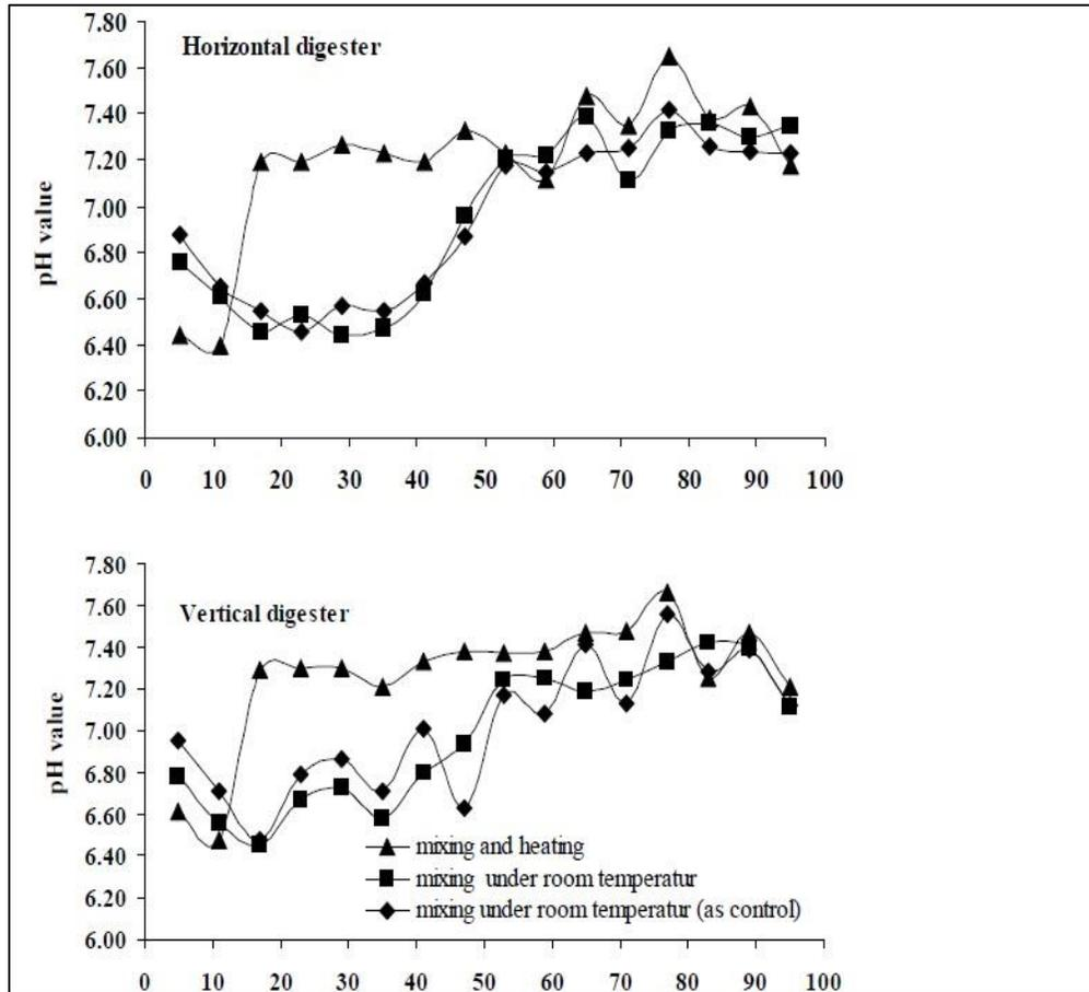
Fig 6: The pH diagram of the yield of two digesters with different mixers[1].
