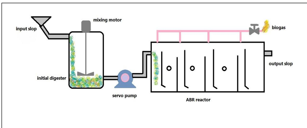
Figure 1: Developed ABR Reactor with Primary Complete Mixing
