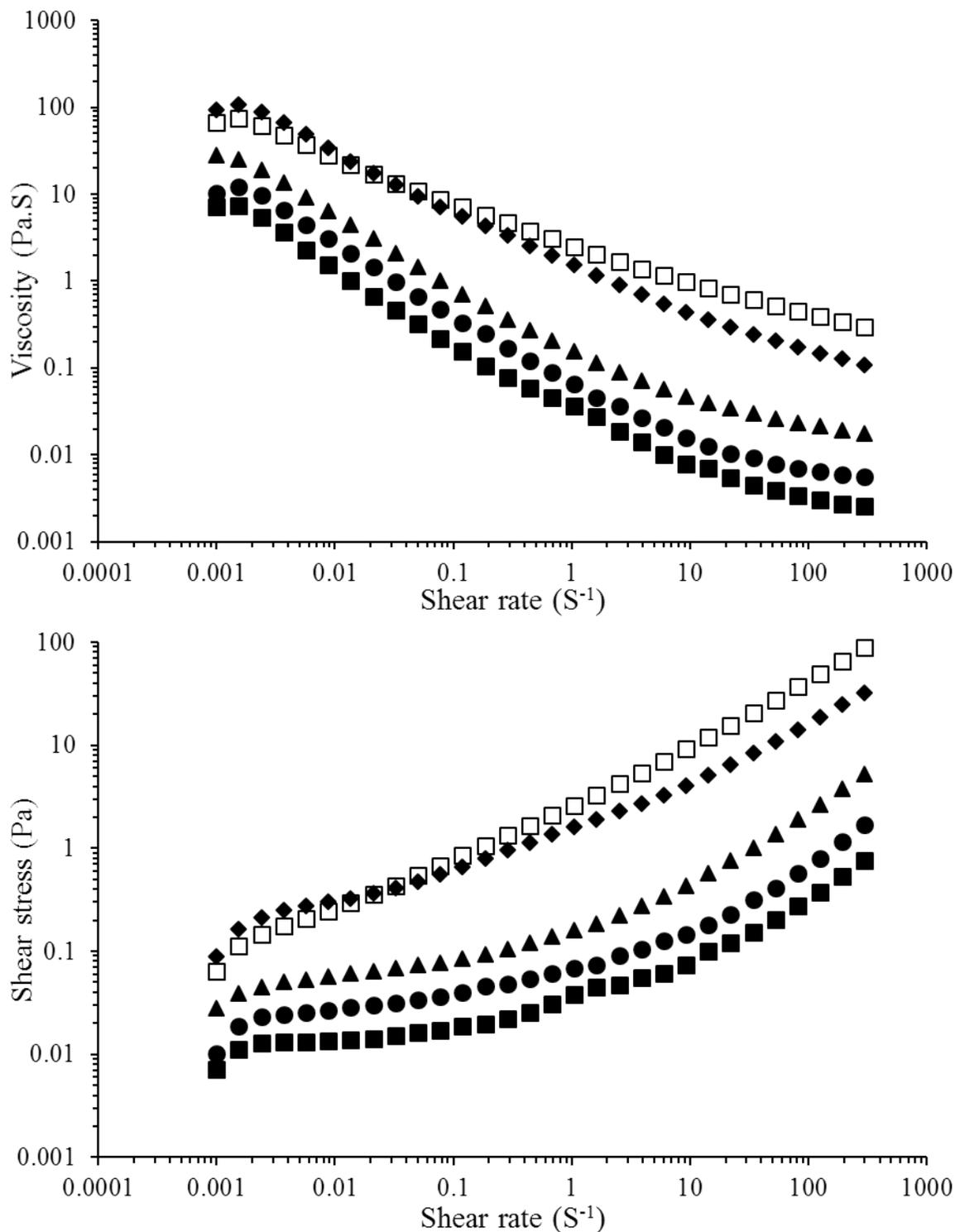
**Fig. 3:** The viscosity and shear stress curves of grapefruit juice and concentrates at different shear rates at 25°C (■: °Brix 9.5; ●: 22 °Brix; ▲: 34.5 °Brix; ◆: 47 °Brix; □: 59.5).
