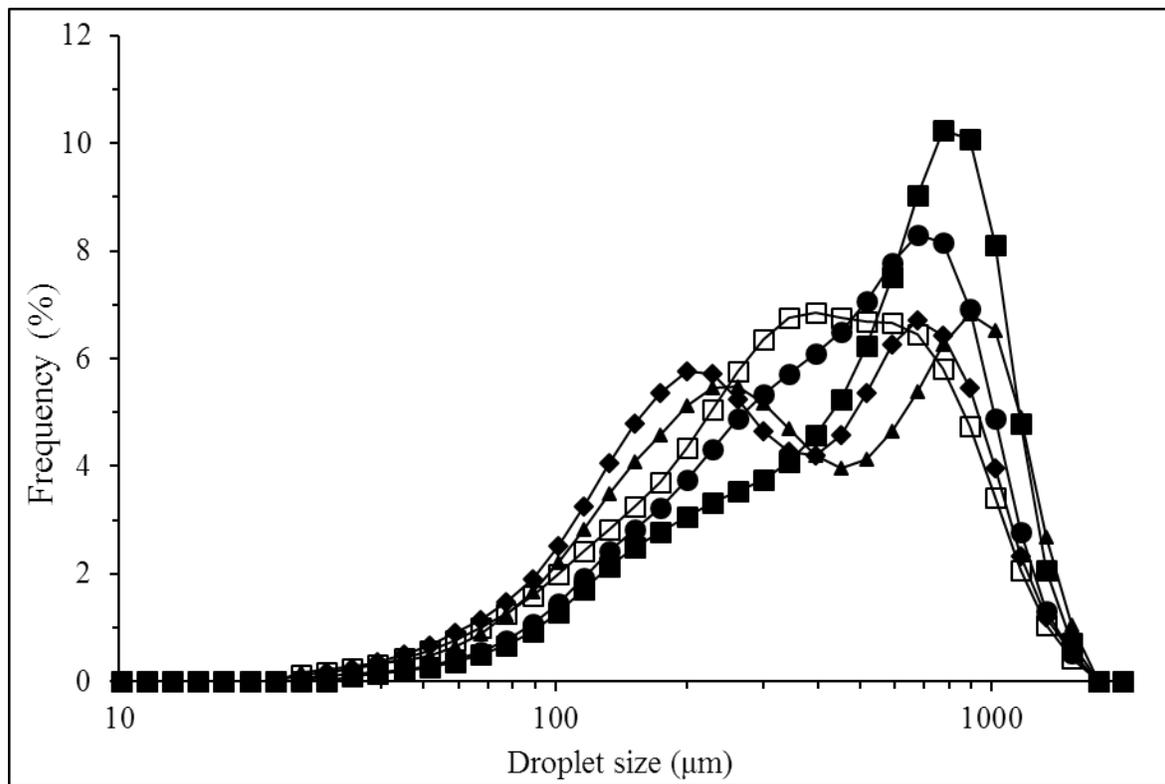
**Fig. 1:** Particle size distribution curves of grapefruit juice and concentrates (■: °Brix 9.5; ●: 22 °Brix; ▲: 34.5 °Brix; ◆: 47 °Brix; □: 59.5).
