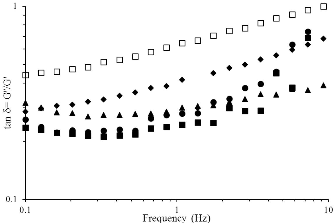
**Fig. 5:** The frequency sweeps of grapefruit juice and concentrates based on  $G^*$  and  $\tan \delta$  in function of the frequency at 25°C. (■: °Brix 9.5; ●: 22 °Brix; ▲: 34.5 °Brix; ◆: 47 °Brix; □: 59.5).
