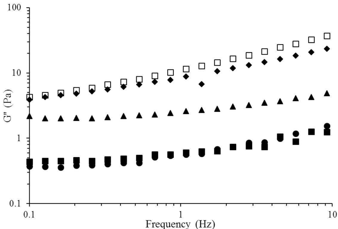
**Fig. 4:** The frequency sweeps of grapefruit juice and concentrates based on storage modulus ( $G'$ ) and loss modulus ( $G''$ ) in function of the frequency at 25°C. (■: °Brix 9.5; ●: 22 °Brix; ▲: 34.5 °Brix; ◆: 47 °Brix; □: 59.5).
